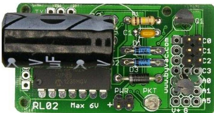
The capacitor can go either up, left or right. When it is laid down like shown it des save some space. The leads need to be soldered so this can happen:
