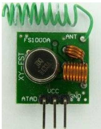
TX module with antenna attached
