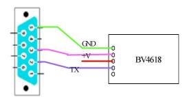
The above shows a connection to an RS232 interface. Power will be needed form an external source and depending on the host internal connections on the 9 pin connector may be required. A typical circuit is:
