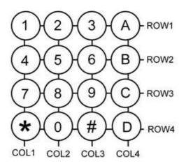
A typical keypad would have the rows and columns connected as indicated on the PCB. The rows are in fact inputs that will be high if not connected to anything. The columns are outputs and are continually being scanned.
