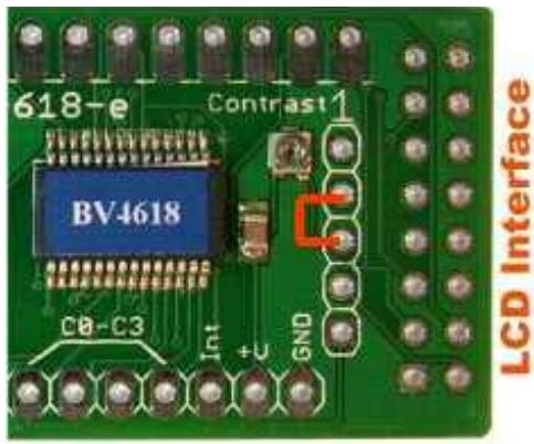
The purpose of the hardware reset is to reset the EEPROM back to a known position so that the display will work correctly. The procedure is:
