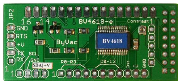
**BV4618****Dual Interface LCD Display & Keypad Controller**
