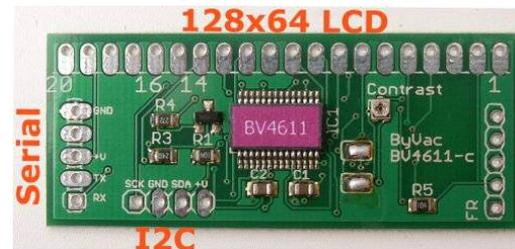
The device has a connector that can either be used for serial or I2C. This is user selectable option, see the section on I2C for more details.
