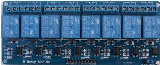
This is an 8 way relay with 10 connections, two are for the supply and the other 8 are for connecting to a controller. When left unconnected or high the relays are off, when a relay pin is connected to ground the relay comes on.
