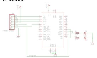
Two LED's are used as status indicators the one marked IND will flash at various rates depending on the status. The one marked PR will illuminate when a connection has been made to another Bluetooth module.
